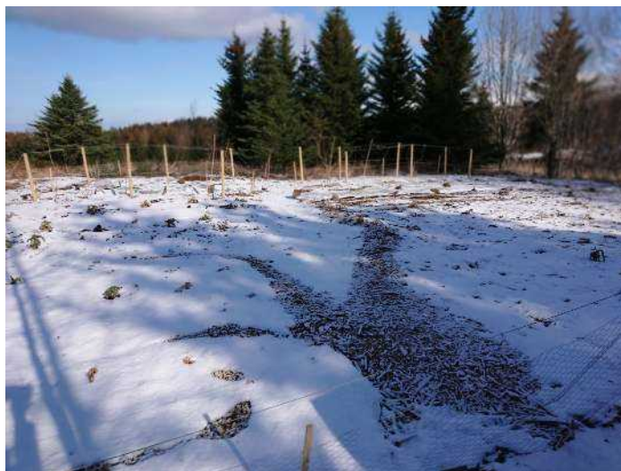
Fig. 18: The garden frozen after the spring planting. Paths of heating tubes are visible in the patterns of melt.
